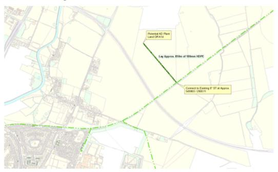
The connecting pipeline of 850m of 180mm High Density Polyethylene has been designed to maintain an acceptable velocity and an acceptable pressure drop (<10mb) for an Entry Connection with a source pressure (Bio-methane injection point) of between 3.5 – 7barg.
